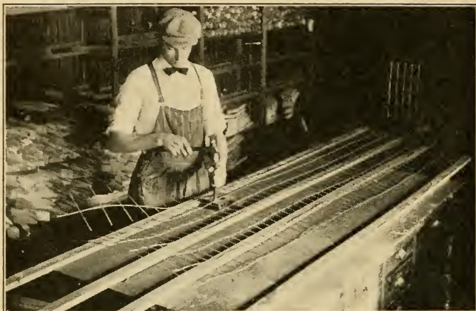
Making seed corn hangers out of electric welded fence. Note the alternate wire method of cutting.
